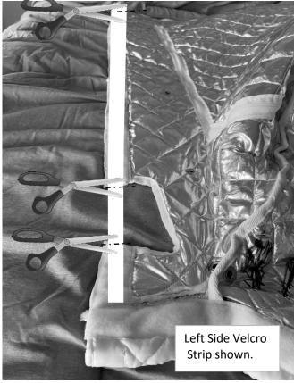
**Mark Velcro Location**: With the straps now attached, grab the Liner by the Velcro, starting in the middle and working out to the corner, Pull the liner tight and mark the location for the top strips of velcro under the cabinet or on the wall next to were the canvas attches.
